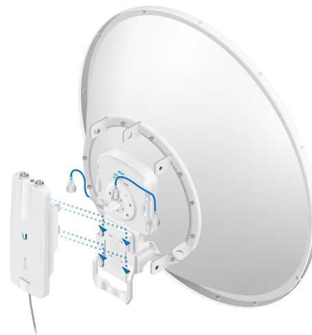
Mounting the AF-11FX on the AF-11G35
